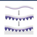
This disc has a paper carrier, designed to create a varied scratch pattern for optimal cutting performance, enabling aggressive sanding and fast material removal.
